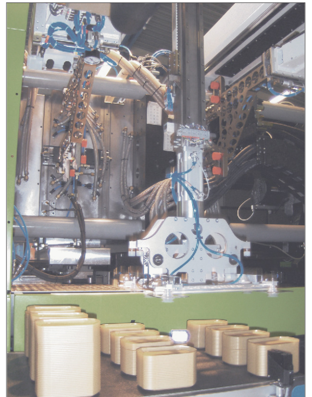
Stack mould automation. In this case, a side robot with a double y-axis. When stacking, the mould impression numbers are not all mixed together but are separated into each type.
