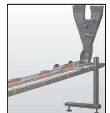
Chute and conveyor for a dual mould take-out system.
